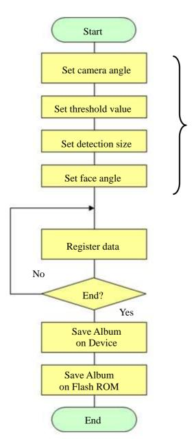
← Change settings as required before registering data (this step is not required if using the default values)
